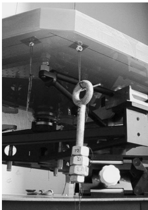
Figure 6. Load being applied to mirror segment
