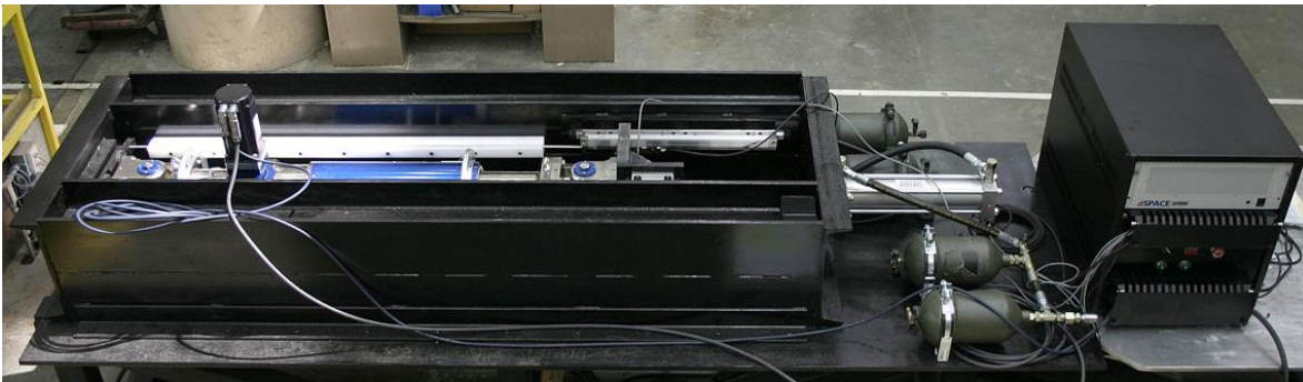
Figure 6. One of the hexapod actuators shown being characterized in a special purpose test stand. Testing of the command v . measured position allowed controller gain tuning resulting in 0.75\mu\text{m} RMS following error at 1\text{mm/s} velocity, which is typical for guiding. Full load testing of the actuator over the 300\text{mm} range of motion resulted in reduction of positioning error from 40\mu\text{m} to less than 5\mu\text{m} .
