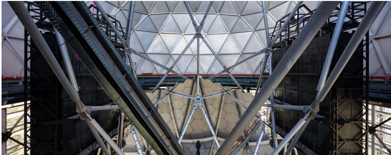
Figure 6: View of the HET from the front showing the primary mirror and the large VIRUS enclosures either side of the telescope structure. They sit on the VIRUS support structure (VSS), which moves on air bearings to follow the azimuth setting of the telescope. The phase separator tanks of the VIRUS Cryogenic System (VCS) can be seen mounted to the top of each enclosure.
