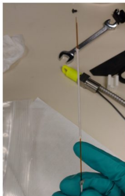
(a) Fiber glass jacketing used to protect fiber
