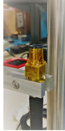
(b) RG695 lens glued on top.
