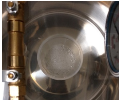
Figure 17: De-gasing the epoxy in a vacuum chamber
