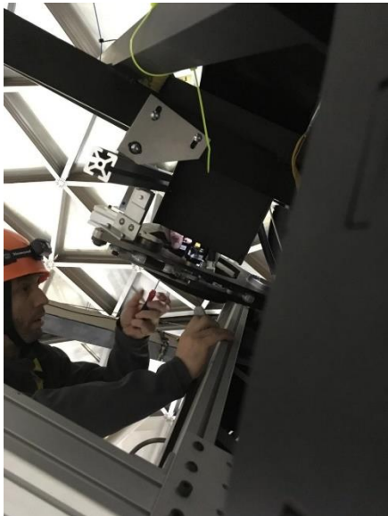
Figure 11. Left photo shows access to the bottom of the input head plate when mounted to the work platform
