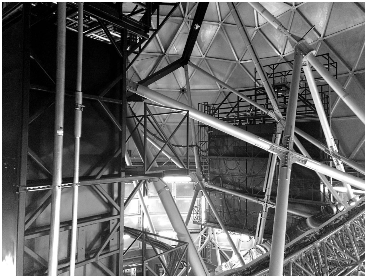
Figure 4. HET with VIRUS enclosures and nitrogen system in place. (Photo taken by R. Spencer)
