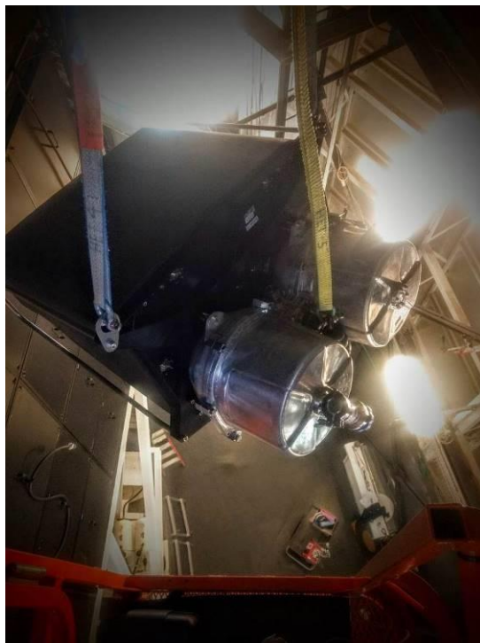
Figure 14. A VIRUS unit being lifted to its assigned enclosure. The 2 gray straps are carrying all the weight. The yellow strap is used in case of lost balance. (Photo taken by R. Spencer)
