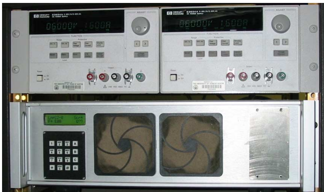
Figure 3. SCS controller front panel. Manual override switches are housed behind the aluminum panel on the right.
