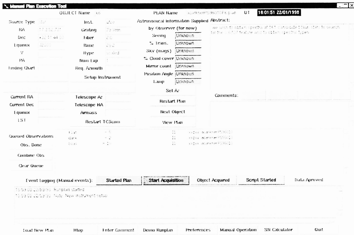
Figure 4 – Our initial plan execution tool. This tool both informs the resident astronomer of what needs to be done as well as creates scripts to be executed by the instrument control system once all manual setups are taken care of. The scientific abstract for the project and any additional comments the PI intends for the resident astronomer to read are displayed. Finally, a list of queued calibrations that are needed to complete this and any previously executed plans are displayed as a reminder of what must be done to complete all open plans. From this interface, the resident astronomer can go into a manual operations mode to run the instrument directly to examine instrument performance or to alter the way a plan is executed.
