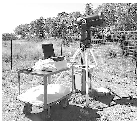
Figure 4 DIMM 2 with computer and CCD. Equipment cart used to transport system to DIMM "pen" each night.
