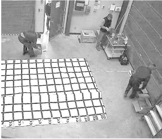
Figure 7: Weather curtain (back side) prior to mounting, showing cargo net sewn to vinyl curtain.
