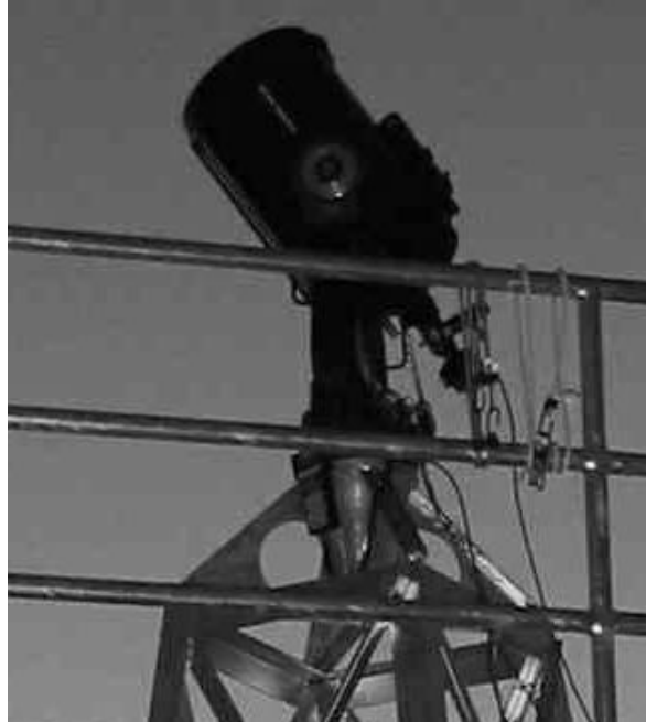
Figure 12: A weldment assures a stiff interface between the tower and telescope. Photo taken during seeing testing prior to dome installation.
