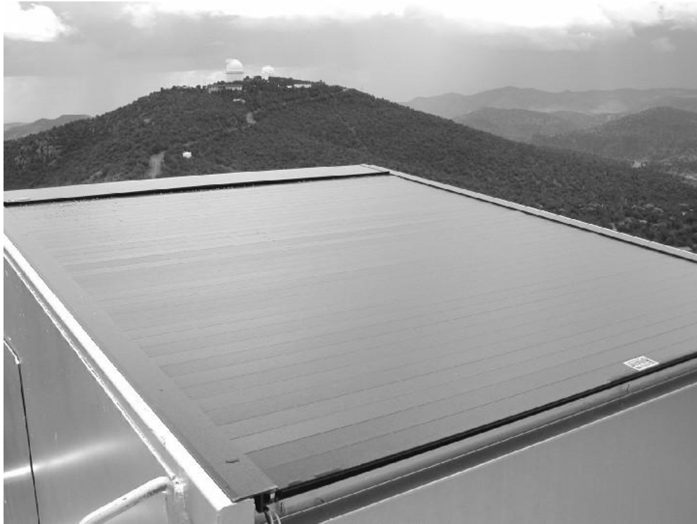
Figure 9: HET DIMM enclosure with roof shutter (Pace-Edwards pick-up bed cover) closed.
