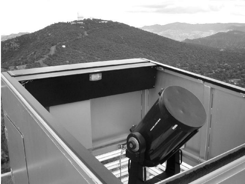
Figure 8: HET DIMM enclosure with roof shutter (Pace-Edwards pick-up bed cover) and louvers open.
