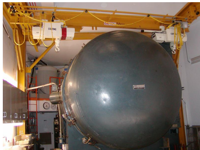
Figure 14. The 2.7-m vacuum chamber with the new 4-ton hoist.
