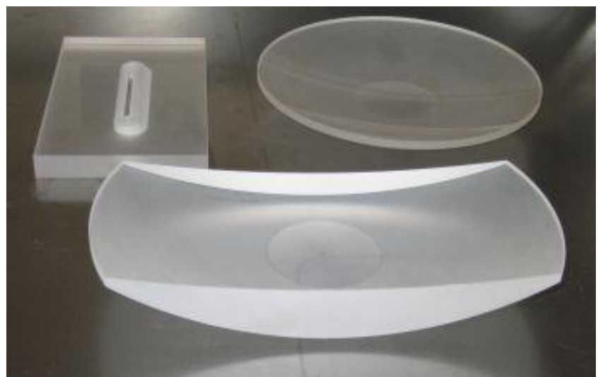
Figure 2: Reflective optics of VIRUS-P prior to coating with high reflectivity dielectric mirror coating. For scale, the collimator mirror in the foreground has a width of 300 mm. The flat mirror folds the collimator and has a recess to allow the fiber output pseudo-slit to be arrayed close to the reflective surface of the mirror, minimizing the obstruction of the slot in the mirror. The collimator mirror and camera mirror (rear right) have spherical backs to minimize weight, and were optimized with finite-element analysis to minimize weight. Flats on their rear sides will be bonded to Invar disks for mounting. All substrates are fused silica.
