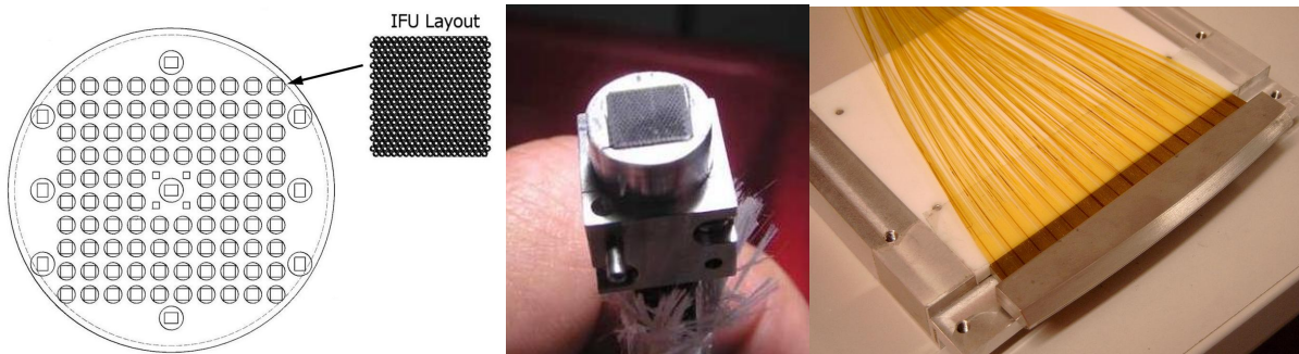
Figure 9. The illustration on the left shows the IFU arrangement at the WFC focal surface. The center photograph is a closeup of a VIRUS-P input head which contains 246 fibers. The photograph on the right illustrates how the fibers are "fanned out" into a linear array at a VIRUS-P output head.
