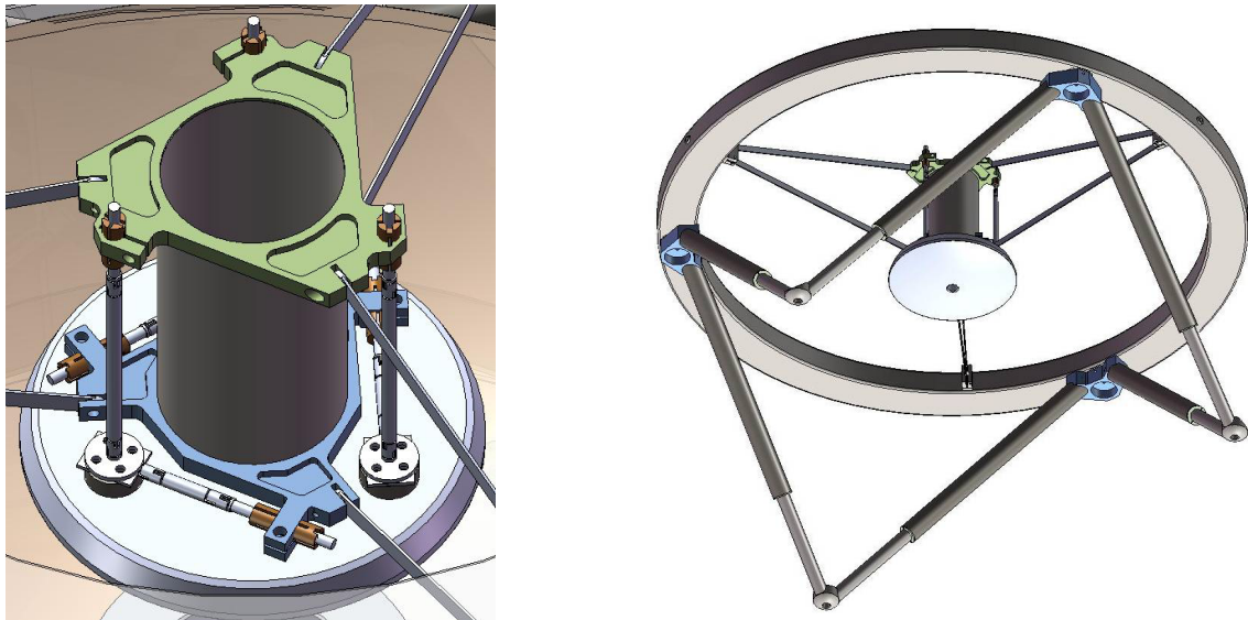
Figure 10. The small convex mirror, M4 is supported at three points. Connections via 6 flexures are made from these points to the M4 support structure, which is held by six tensioned vanes to a headinging. The headinging is supported by 6 truss tubes
