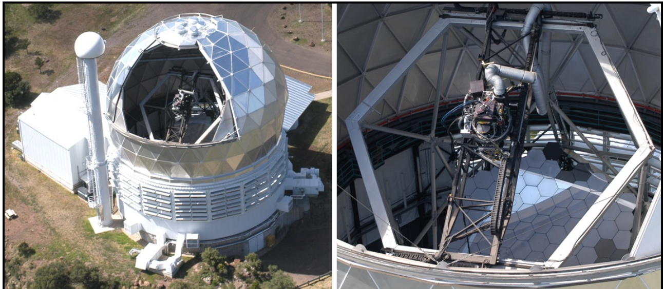
Figure 1. The figure on the left shows the HET pre WFU with the dome shutter open. The figure on the right is a close up view of the top of the HET revealing the primary mirror, and telescope structure which supports the tracker and PFIP.
