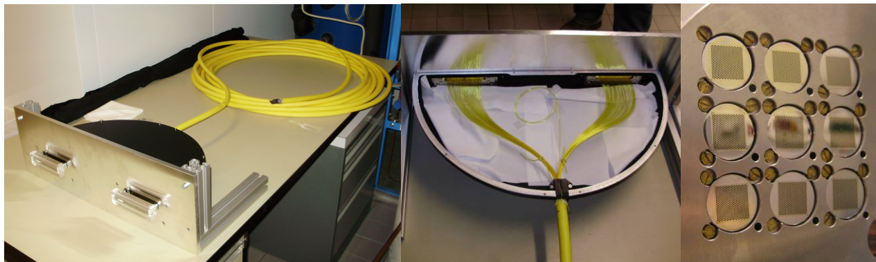
Figure 6. Production IFU cables at AIP. Left and middle images show the slit assembly with the two slit blocks that feed the pair of spectrographs within a VIRUS unit. The slit assembly mounts to the collimator kinematically. The cable length is 22 m. Right shows nine IFUs input heads mounted as they will be at the HET focus. Three screws and a pin locate the heads. AR coated cover plates are not yet applied in this view. The heads have a ¼ fill-factor in the field of view. This configuration provides the ability to fill in the field of view by offsetting the telescope to four positions.
