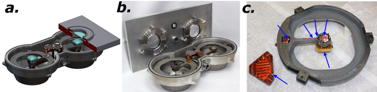
Figure 10. Assembly for integrated testing of camera pair cryogenics. a) Solid model of the integrated test assembly showing the large vacuum plate with windows installed cut away, revealing internal components. b) A photo of the integrated test assembly and vacuum plate. c) A photo of the spider with installed cryogenic components showing the location of the various RTDs ( blue arrows ) used for testing \Delta T across component junctions.
