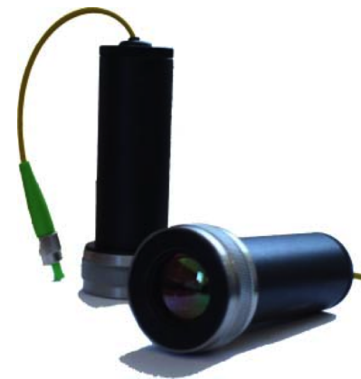
Figure 4 The DMI measurement heads with a focusing lens at the output end of the head [7] .
