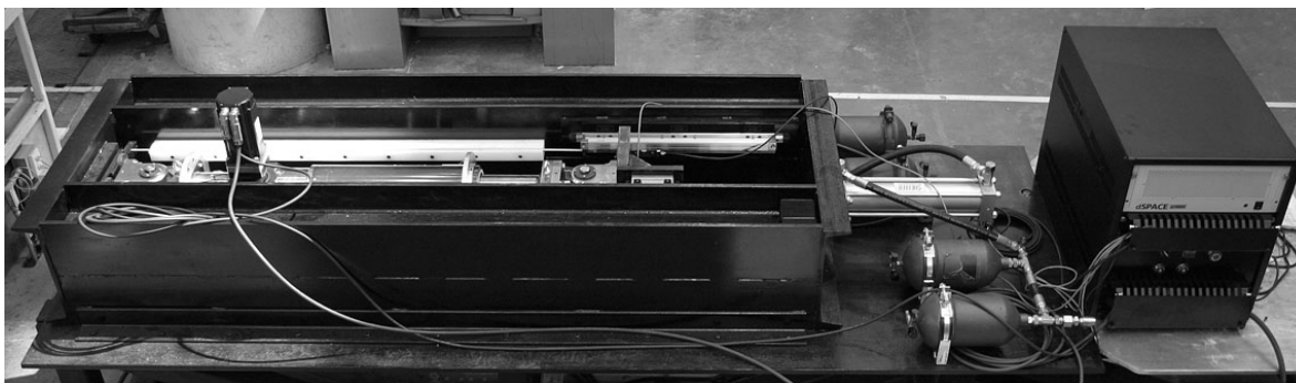
Figure 4. Prototype actuator for the hexapod shown mounted on the test bench at CEM.
