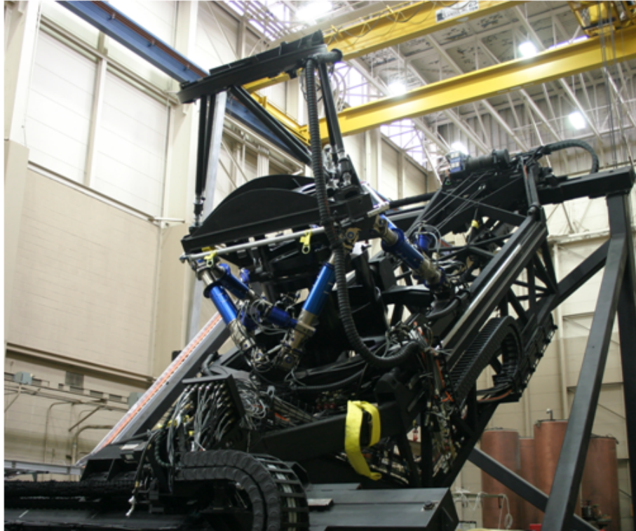
Figure 13. Current configuration of the HETDEX tracker system
