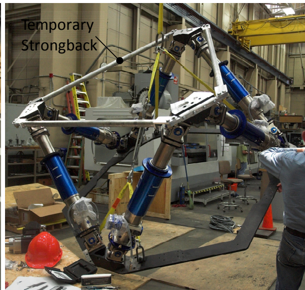
Figure 7. Temporary strongback installation; 35 degree lift
