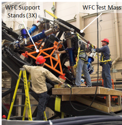
Figure 11. WFC test mass installation
