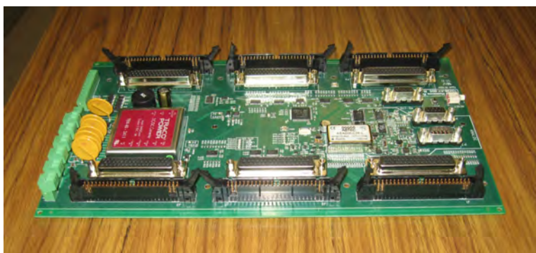
Figure 13. Hardware fault controller prior to installation in HETDEX control rack.
