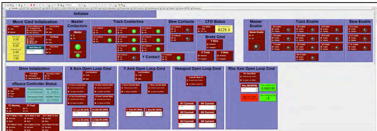
Figure 11. Screen capture of 1 page of dSpace “Control Desk” Tracker controller Graphical User Interface
