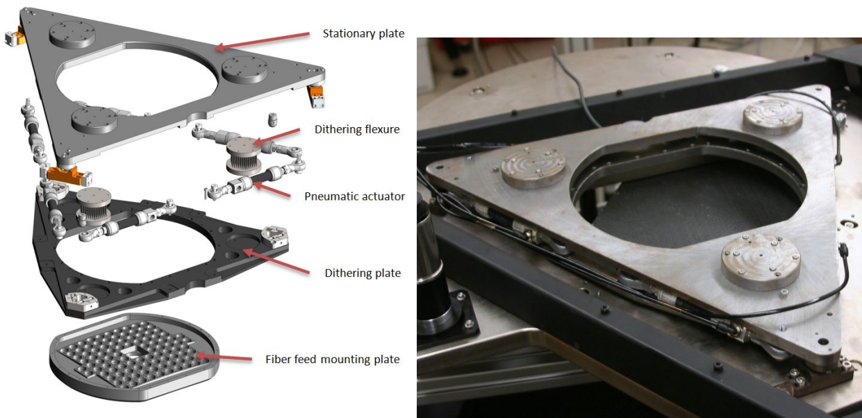
Figure 14, left shows an exploded rendering of the dithering mechanism and the fiber feed mounting plate. Figure 15, right shows a photo of the dithering mechanism and shutter underneath.
