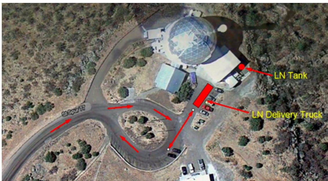
Figure 11. Google Earth view of the HET facility showing LN delivery truck maneuvering room at the telescope. The 11,000 gallon vacuum jacketed tank is located at the rear of the facility as indicated with fill tubes extending to the HET car park.
