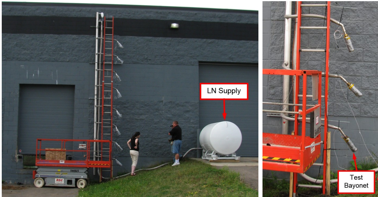
Figure 12. Functional performance test setup of VCS components at Midwest Cryogenics. Right is a close-up view of some of test bayonets that were used to simulate the heat load imposed by VIRUS. Left gives a sense of the scale of the system.
