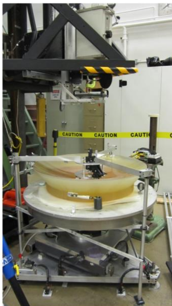
Figure 9. Photo of the center reference fixture registration under optical test and centration calculation by coma measurement of M5
