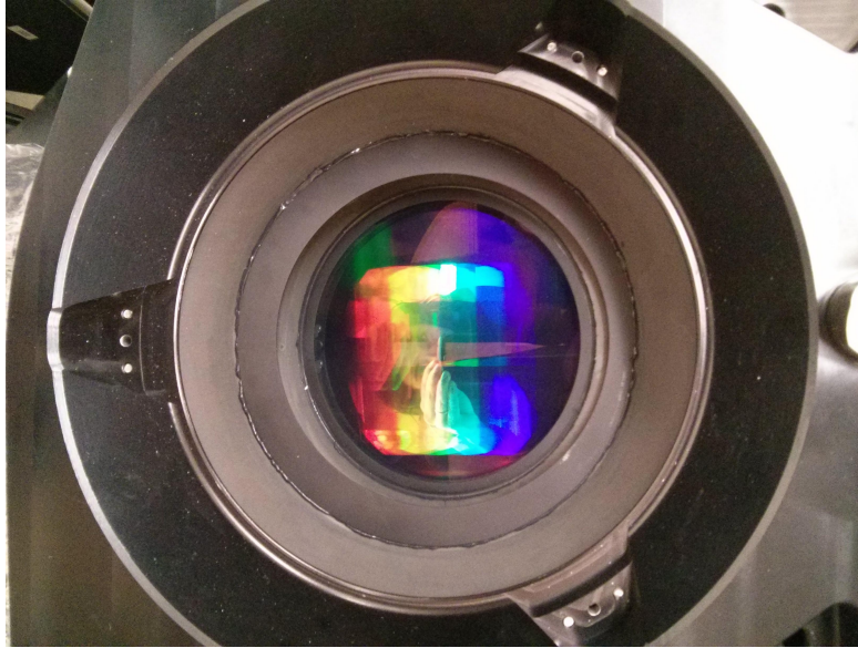
Figure 4: An image of one VPH grating mounted in its cell, and then in the collimator.
