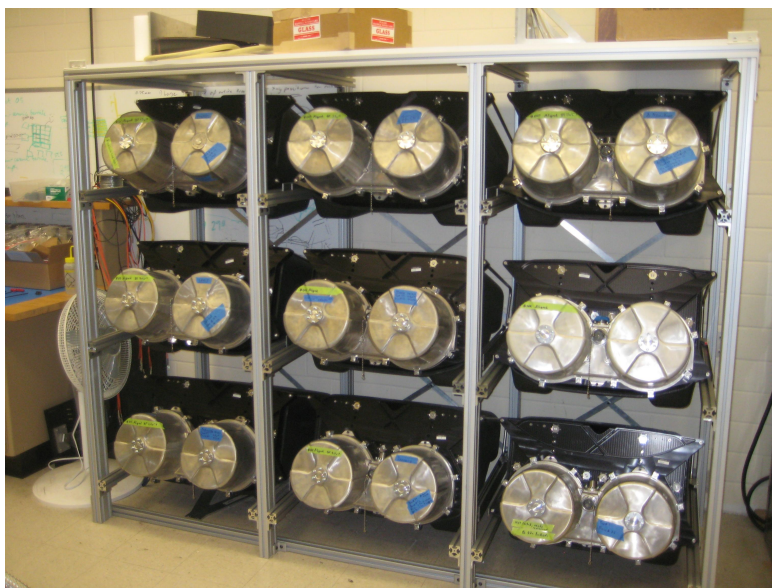
Figure 2: Nine spectrograph units, aligned and stored at the University of Texas at Austin.
