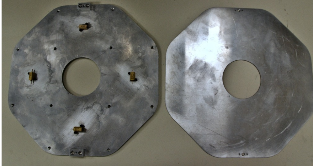
Figure 5. Aluminium panel heater with Vishay resistive heaters and protective cover. The Vishay heaters are mounted to the panel using indium foil to enhance thermal contact.
