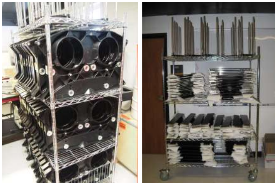
Figure 6. Collimator subassemblies were pre-assembled and stored before the final collimator assembly. Shown here are the base plates (left) and side, top, and bottom plates (right). Each of these components has multiple alignment and attachment features to facilitate the final assembly. Collimator mounting plates with attached Invar metering rods can be seen on the top rack of the carts.
