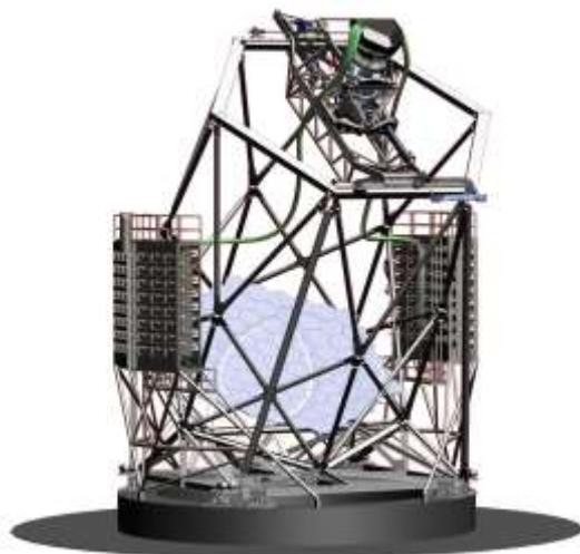
Figure 1. The VIRUS spectrograph pairs will be mounted inside two climate-controlled enclosures located on either side of the telescope.
