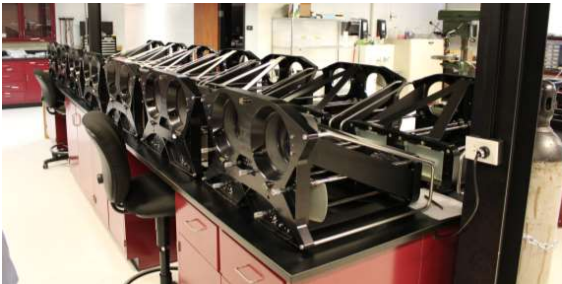
Figure 7. Collimators were completed in batches of 10-15 at a time. This number was primarily set by the size of the assembly bench. Each set of 10-15 collimators were assembled over a 2-3 week period.
