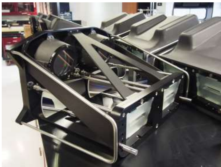
Figure 8. One complete collimator with all optics installed. Additional completed collimators (with their protective covers installed) may be seen in the background.
