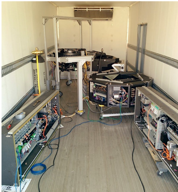
Figure 19. The FPA instrumentation and electronics setup in the refrigerated truck for cold testing
