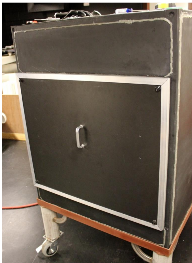
Figure 6. The enclosure door design installed on the enclosure prototype to test the amount of pressure it can hold with varying flow rates.
