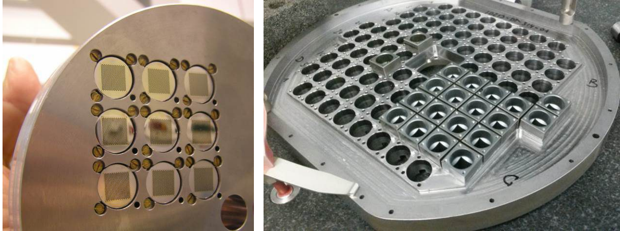
Figure 9. Left: a first configuration of 3 \times 3 IFUs mounted in a preliminary plug plate, featuring over 4000 fibres. Right: The complex and precise Input Head Mount Plate (IHMP, produced at IAG) allows to accurately position up to 96 VIRUS IFUs in a rectangular grid with a \frac{1}{4} fill factor and with spherical curvature that matches the telescope focal plane.
