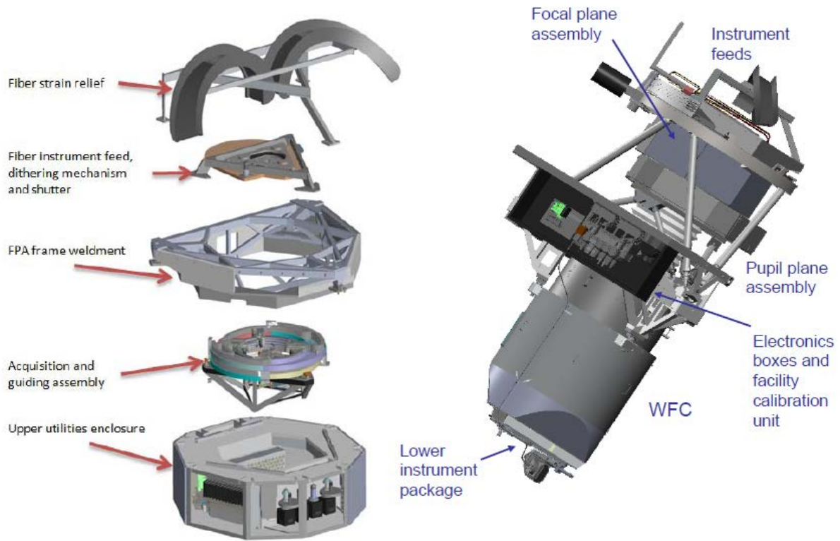
Figure 6. Renderings of the PFIP. On the right the full assembly is shown with major sub-assemblies indicated. On the left is an exploded view of the FPA showing its major components. The FPA contains most of the complexity of the instrument, including the acquisition and guiding (AG) assembly with guide probes and wavefront sensors.
