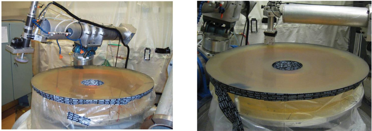
Figure 2 On the left is shown the robotic computer controlled grinder/polisher. The machine incorporates a Swing arm Optical CMM (SOC) shown on the right, which makes in situ profile measurements at several clocking angles of the part that later synthesized to estimate a two dimensional figure map. Two such machines are used; one machine performs initial shaping and polish out with high-speed grinding/polishing spindle and optical probe that measures diffuse reflections; the other machine performs final figuring with pitch laps, guided by a high performance SOC that incorporates an interferometric sensor.
