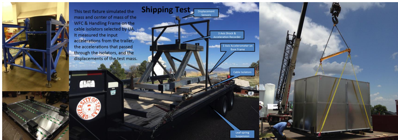
Figure 18 The shipping container of the WFC system. (Top left) the complete WFC system at the transportation orientation within its maintenance cart. (Bottom left) the shipping base with cable shock isolators. (Middle) The mock-up shipping test to verify the cable isolator performance. (Right) the delivered shipping container with the WFC inside at the HET parking lot with a crane lifting the assembly to load into the HET receiving bay.
