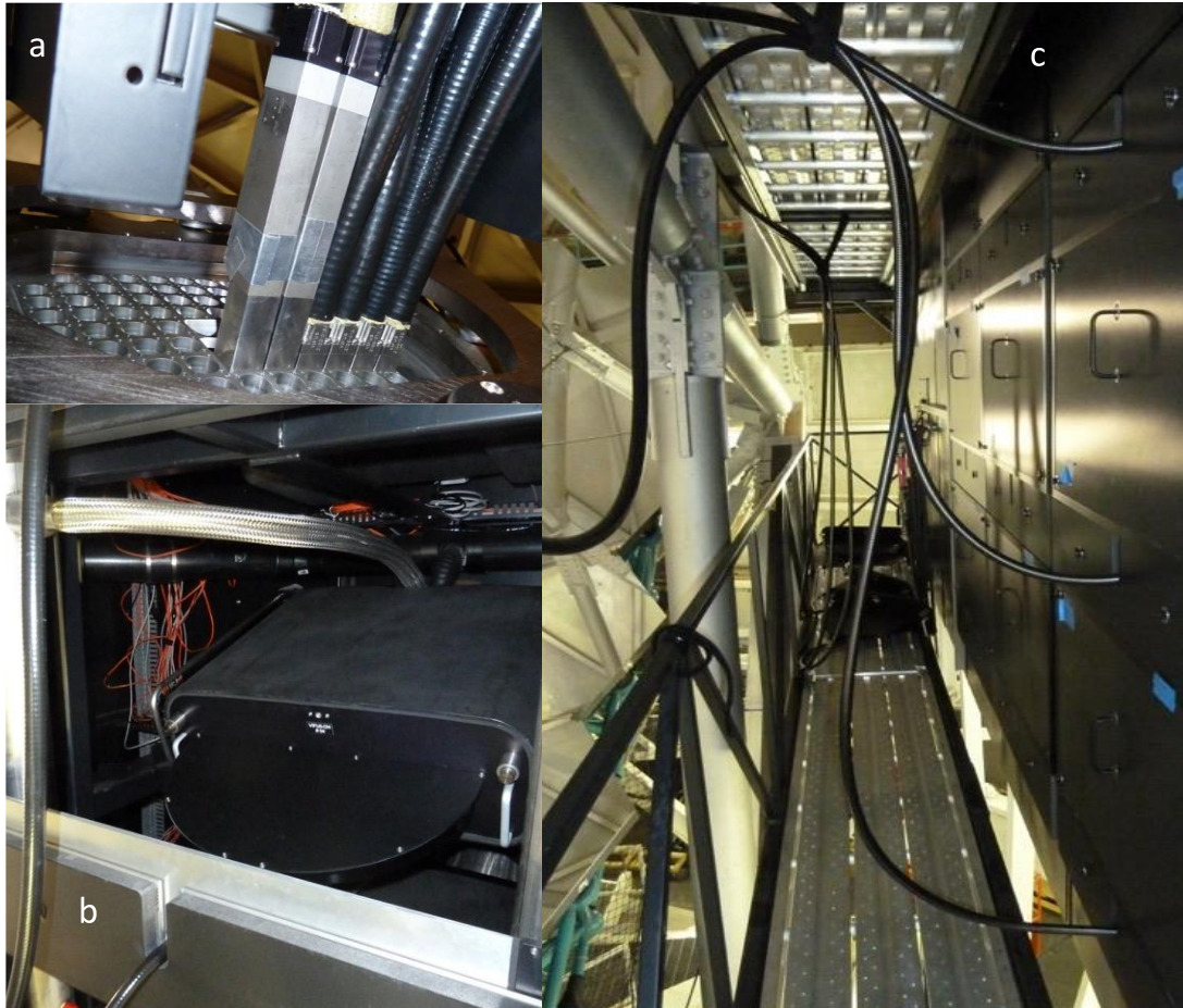
Figure 10: VIRUS IFU deployment (a) 16 VIRUS IFUs (black conduit) and the two LRS2 IFUs installed in the input head mount plate (IHMP) at the prime focus of the HET; (b) IFU tailpiece installed on a VIRUS unit in the enclosure, note the stainless steel braid on the liquid nitrogen “dogleg” cooling the spectrographs; (c) VIRUS enclosure sealed up after IFU installation.
