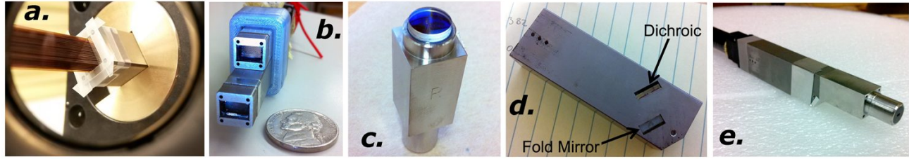
Figure 11. Assembly of the LRS2 IFU inputs. a ) Feeding fibers through the hole block by Berlin-Fibre GmbH. b ) The LRS2-B input heads. The nickel is shown for scale. Individual lenslets can be seen. c ) The focal extender subassembly. Doublet 2 can be seen protruding from the end of the lens barrel. d ) The dichroic subassembly housing. e ) A fully assembled LRS2 IFU input assembly.
