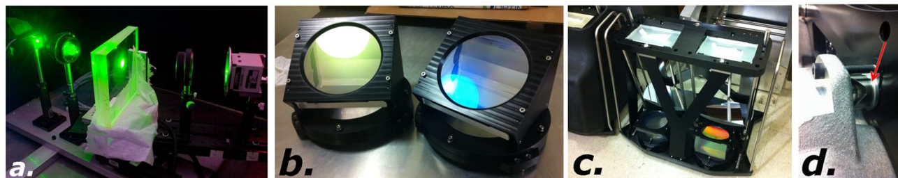
Figure 9. Photos of the LRS2 collimator assembly. a ) The LRS2-B Orange Arm grism under test using the VPH grating test bench that was originally developed for VIRUS. b ) The LRS2-R Red Arm (right) and Far Red Arm (left) grisms installed into their fully assembled mounting cells. c ) LRS2-B's collimator assembly complete, with the plastic cover removed to reveal the internal optics. d ) Arrowed is one of the collimator vee-block shims that are used to fine-tune the camera-collimator angle to compensate for the delivered G_{\Lambda} values of the grisms.
