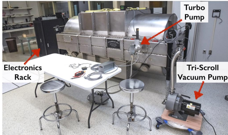
Figure 3. The HPF cryostat during long-term stability testing. The scroll and turbo pumps are only used during initial vacuum pumpdowns. They were turned off during long-term stability testing, leaving the charcoal getters and NexTorr pump to maintaining the vacuum. No additional thermal enclosure was used.
