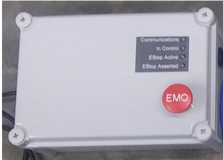
Figure 1. Photograph of a Remote unit showing the user interface, 4 LEDs, 1 pushbutton.
