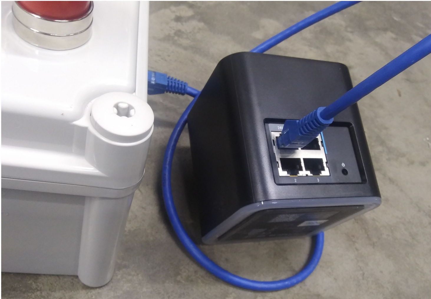
AirCube for Estop Enclosure is powered by POE unit inside of enclosure. Connect Cat5e cable to port labeled '24V POE in'
